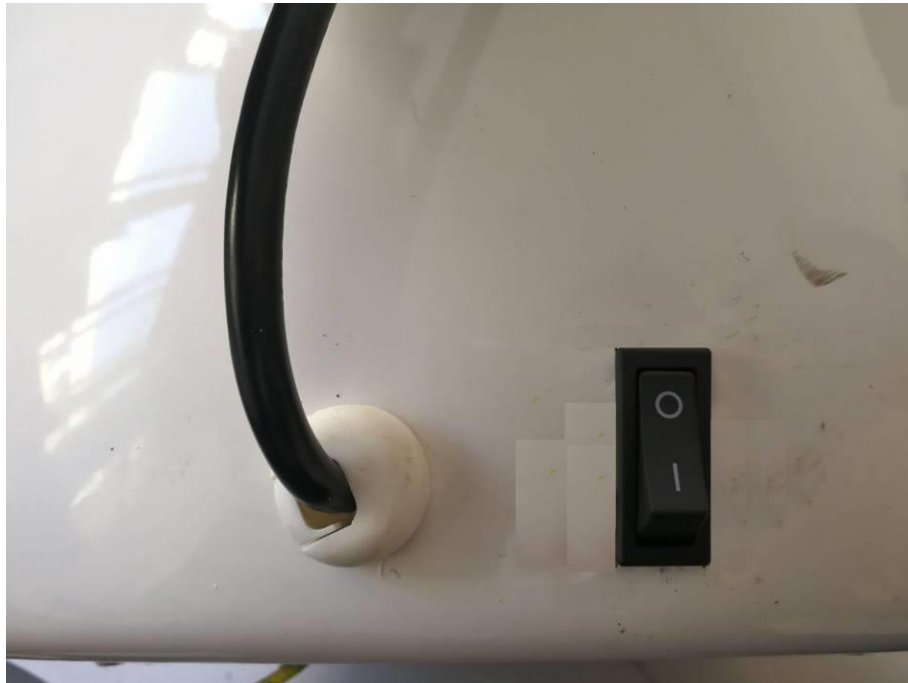
Switch and cord anchorage
